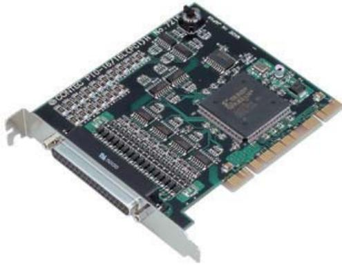
This board is a PCI-compliant interface board for input/output of digital signals.
